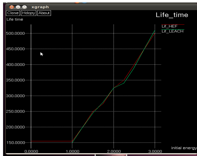
Fig 5. Graph showing comparison on lifetime of Leach and High Energy First Protocol.
